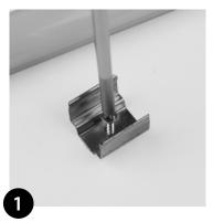
Fix clips securely into suitable surface with suitable screws (Allow 4 per metre/39.4in).
